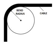
A reduced bend radius fibre is able to withstand tighter bends within frames, panels and pathways. It also enhances the reliability of a network and reduces network down time.
