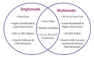
Commonly, singlemode fibre gives a higher transmission rate and up to 50 times more distance than multimode fibre, but it also costs more.
